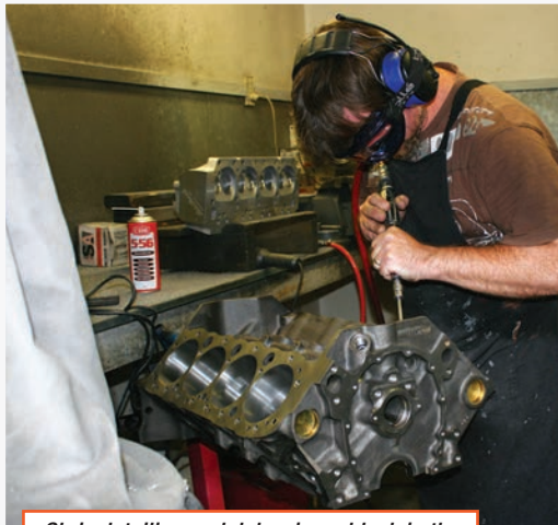
Chris detailing and deburring a block in the porting room. Port matching, cylinder head porting and flow-testing is all carried out on-site and the team know all the tricks!
