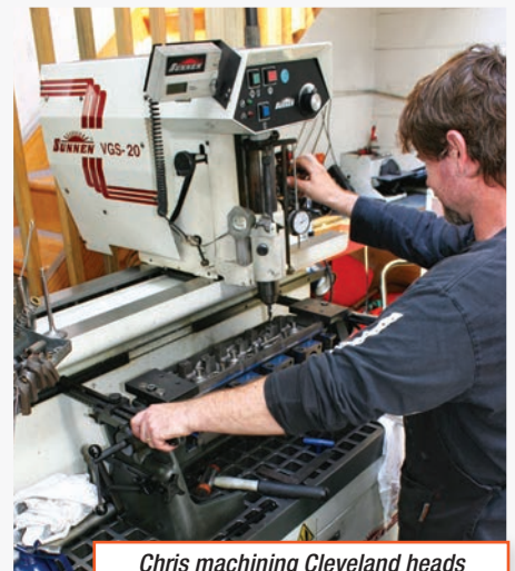
Chris machining Cleveland heads on a Sunnen Head Shop.
