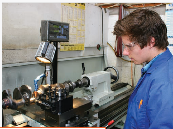
Scott Marsh turning down counterweights for crankshaft balancing.
